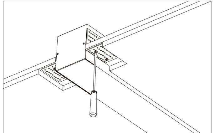
4. Place the profile into the cut-out hole with the L brackets fitting into the small recess made area. Secure L brackets accordingly.
