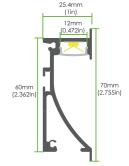
Optional Diffuser (PMMA/PC)
