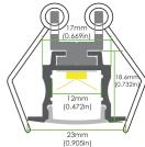
Optional Diffuser (PMMA/PC)
