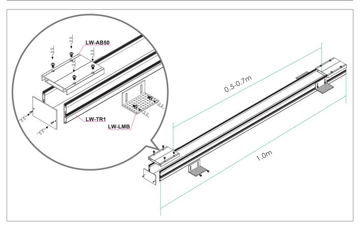
1. Assemble the AB and TR1 into each other as pictured above, followed by the end caps into place. Ensure the AB clamps are placed between 50-70cm apart.
