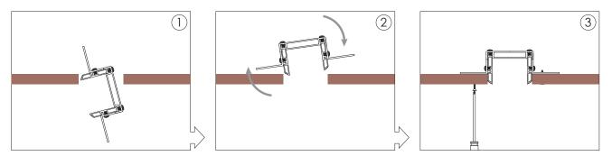
4. Insert the housing sideways into the cut-out hole, then rotate it until it lays flat on the ceiling board. Secure with screws from the underside of the ceiling board (ceiling surface).
