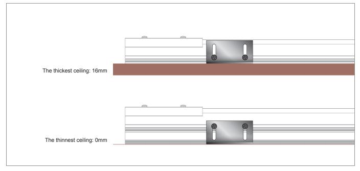
2. Adjust and install the L brackets according to ceiling board thickness.
