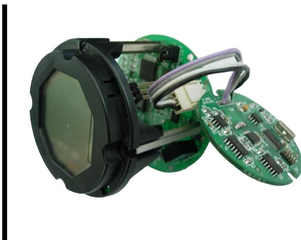
A Board Set for HART Capacitance Pressure Transmitter Board Set
