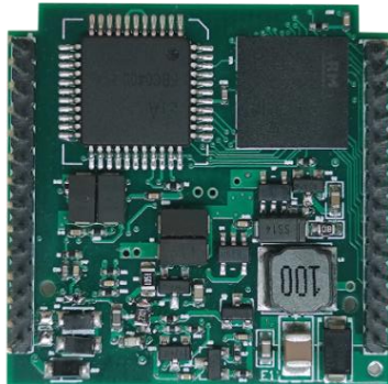
Figure 3 Structure of MC0312 built-in core module
