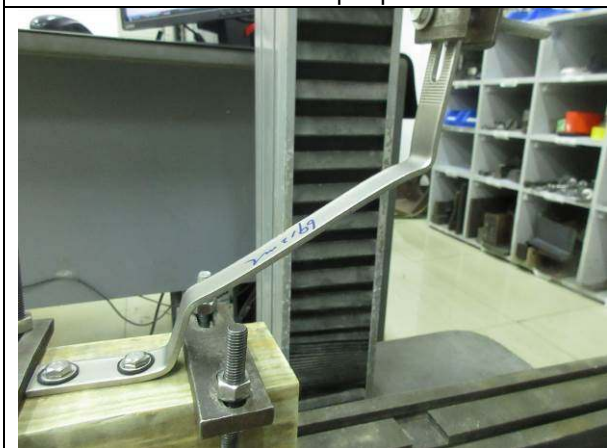
Photo 3: after tensile test (obvious deformation)
