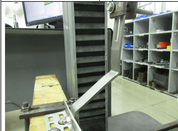
Photo 3: after tensile test (obvious deformation)
