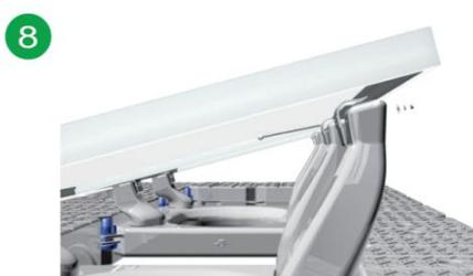
Using Clamp Kit and Screw Kit to fix solar panel on the Back Legs.
