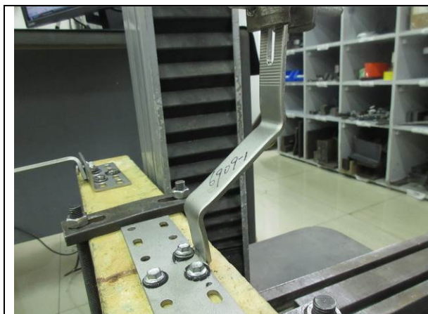
Photo 3: after tensile test (obvious deformation)
