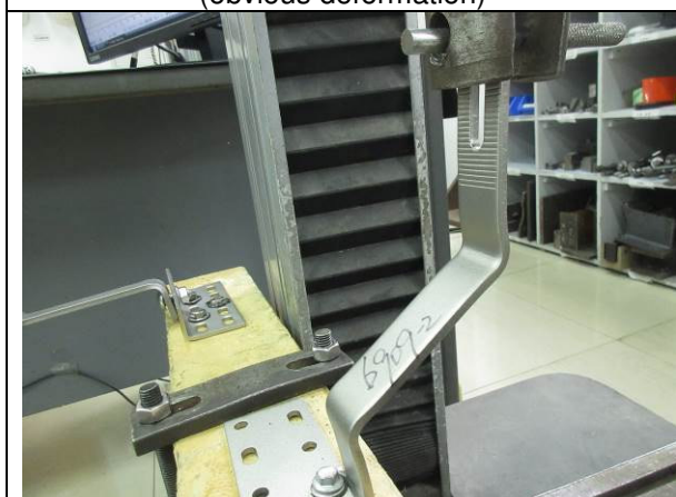
Photo 5: after tensile test (obvious deformation)
