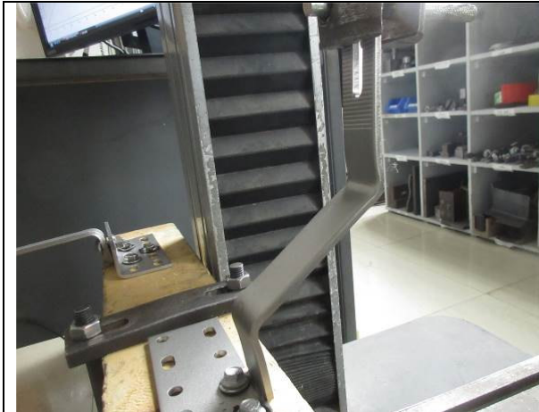
Photo 7: after tensile test (obvious deformation)
