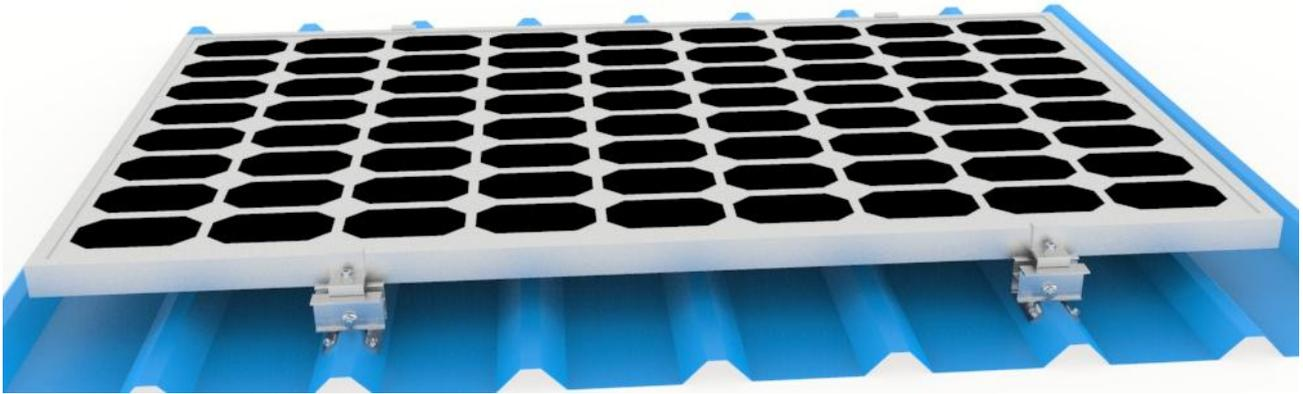
Universal Roof Clamp can work with all kinds of trapezoidal metal roof. It is a rail-less solution, it will help you save some cost and labor cost. Use anti-aging EPDM rubber to improve the waterproof performance. The material of this product is made by aluminum alloy (AL 6005-T5) and stainless steel 304 (SUS 304), which has strong corrosion resistance.
