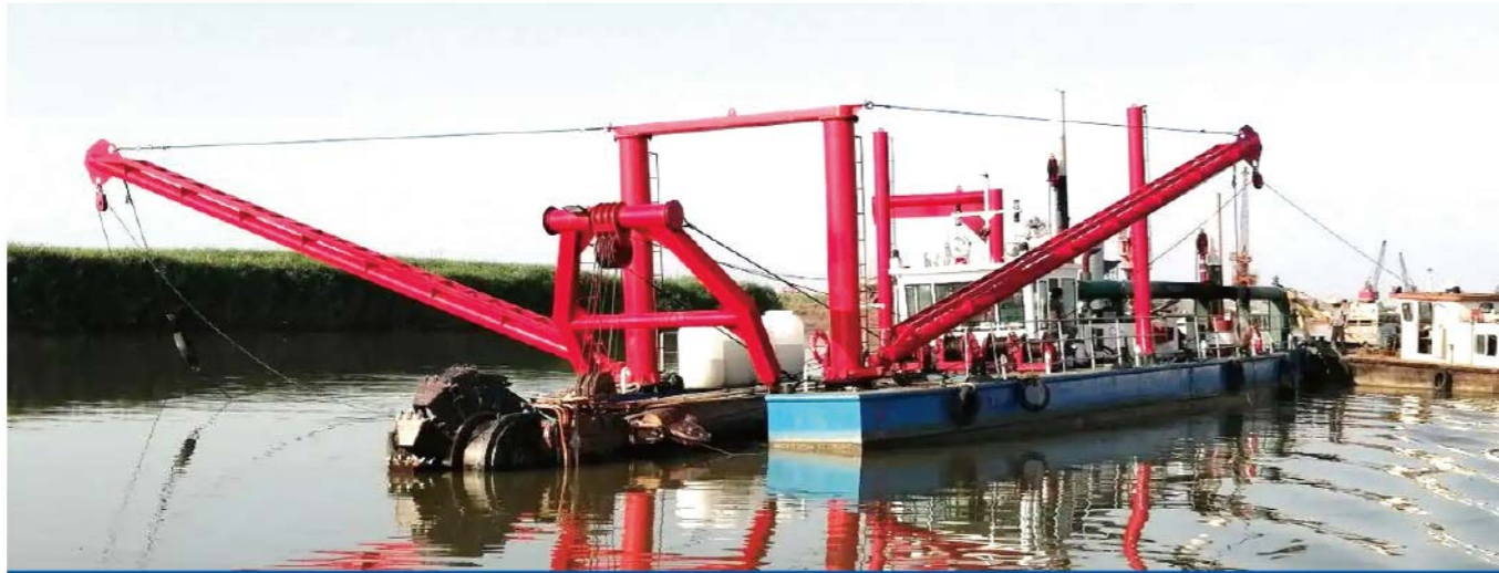
斗轮式挖泥船 Bucket Wheel Dredger
