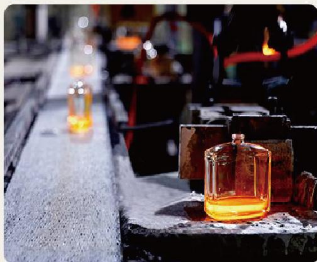
出炉 Discharge from furnace
