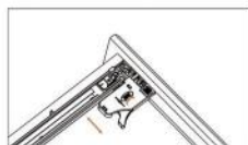
Drawer panel left/right adjustment
