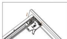
Drawer panel up/down adjustment
