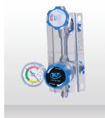
Series: TKF-5-9 Max,inlet Pressure: 1000psi Outlet Pressure Aange: 0-300psi Connection: 1/4"- 1/2"LOK Flow Coefficient: cv= 0.03
