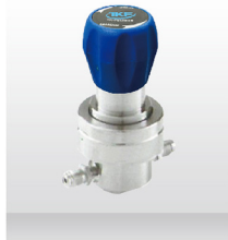
Series: TKF-Re2-2 Max,inlet Pressure: 1000psi Outlet Pressure Aange: 0-300psi Connection: 1/4"M-VCR Flow Coefficient: cv= 0.06
