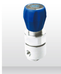
Series: TKF-Re1-3 Max,inlet Pressure: 6000psi Outlet Pressure Aange: 0-2500psi Connection: 1/4"FNPT Flow Coefficient: cv= 0.06
