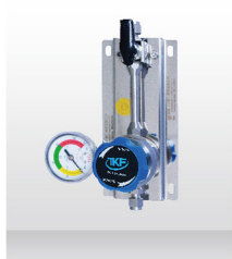
Series: TKF-5-3 Max,inlet Pressure: 1000psi Outlet Pressure Aange: 0-300psi Connection: 1/4"- 1/2"LOK Flow Coefficient: cv= 0.08
