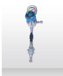
Series: TKF-5-2 Max,inlet Pressure: 1000psi Outlet Pressure Aange: 0-300psi Connection: 1/4"- 1/2"LOK Flow Coefficient: cv= 0.08
