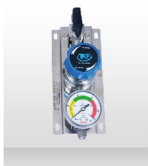
Series: TKF-5-1 Max,inlet Pressure: 1000psi Outlet Pressure Aange: 0-300psi Connection: 1/4"- 1/2"LOK Flow Coefficient: cv= 0.08
