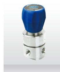
Series: TKF-Re1-4 Max,inlet Pressure: 1500psi Outlet Pressure Aange: 0-160psi Connection: 1/2"FNPT Flow Coefficient: cv= 1.0
