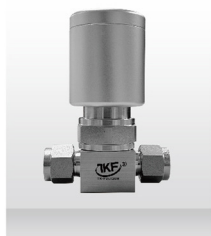
Series: TKF-PV3 Max,Working Pressure: 0-3000psi Actuator Pressure Rating: 0.4-0.7Mpa Connection: 1/4-3/4"LOK Flow coefficient: Cv=0.65
