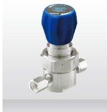
Series: TKF-Re2-1 Max,inlet Pressure: 1000psi Outlet Pressure Aange: 0-300psi Connection: 1/4"F-VCR Flow Coefficient: cv= 0.06
