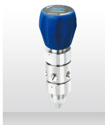
Series: TKF-Re1-2 Max,inlet Pressure: 3500psi Outlet Pressure Aange: 0-1000psi Connection: 1/4"FNPT Flow Coefficient: cv= 0.06
