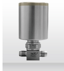
Series: TKF-PV4 Max,Working Pressure: 0-3000psi Actuator Pressure Rating: 0.4-0.7Mpa Connection: 1/4-3/4"M-VCR Flow coefficient: Cv=0.65
