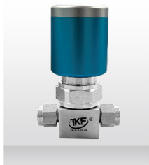
Series: TKF-PV1 Max,Working Pressure: 0-1000psi Actuator Pressure Rating: 0.4-0.7Mpa Connection: 1/4-3/4"LOK Flow coefficient: Cv=0.3
