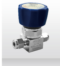
Series: TKF-DV3 Max,inlet Pressure: 3000psi Outlet Pressure Aange: 0-3000psi Connection: 1/4"-3/4"LOK Flow Coefficient: cv= 0.65
