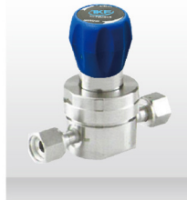
Series: TKF-Re2-3 Max,inlet Pressure: 3500psi Outlet Pressure Aange: 0-1000psi Connection: 1/4"F-VCR Flow Coefficient: cv= 0.06
