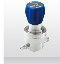
Series: TKF-Re2-4 Max,inlet Pressure: 3500psi Outlet Pressure Aange: 0-1000psi Connection: 1/4"M-VCR Flow Coefficient: cv= 0.06
