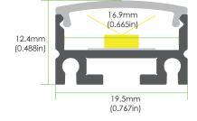
Optional Diffuser (PMMA)
