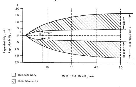
Use of Chart—Calculate the mean test result in minutes. Enter chart at the zero point, A, on the ordinate and move to the right on the abscissa to point B. Compute and locate the deviation points C+ and C-, from the mean test result. If the deviation points fall within the repeatability area, then the results are within the precision of the test.
