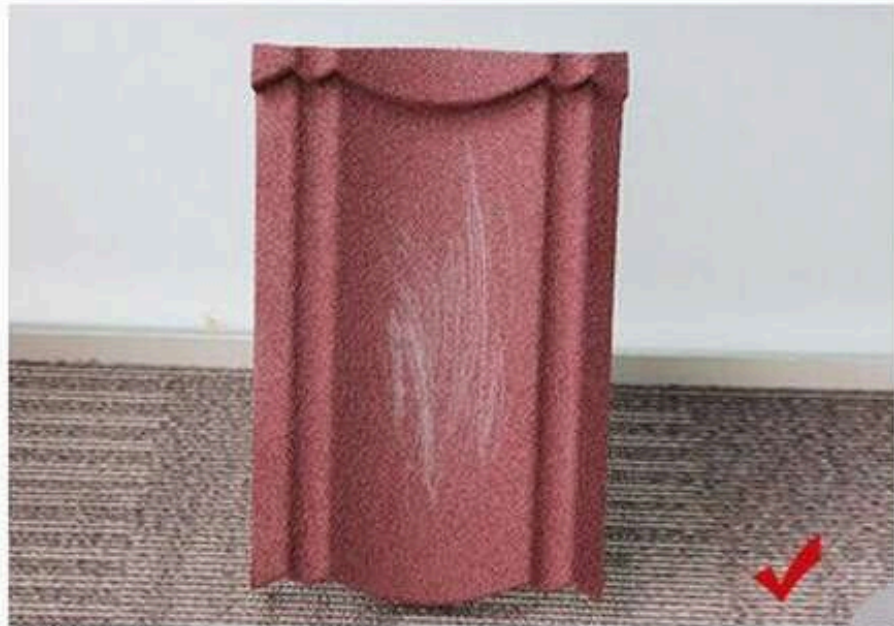
BUILDEX: After Scratch Test
