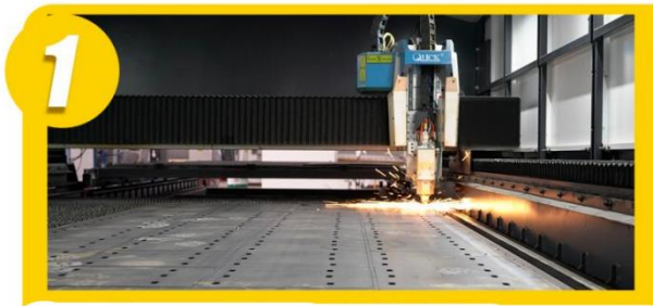
1 数控激光切割，工装精度保证 CNC laser cutting, ensuring tooling accuracy;
