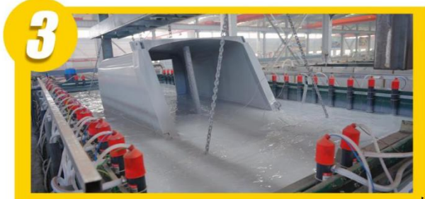
3 顶尖涂装工艺，上装电泳选择，防腐防锈十年无忧 Top coating technology, top electrophoresis selection, worry free anti-corrosion and rust prevention for ten years
