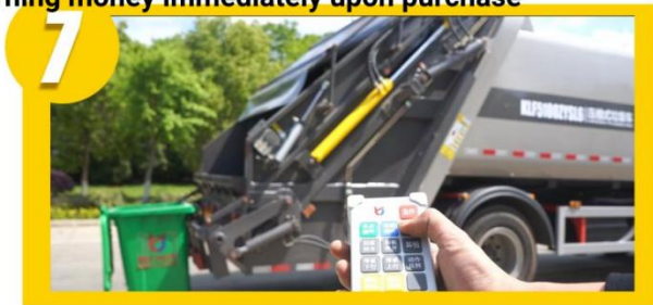
7 电控系统与国外技术团队合作研发，CAN总线控制，相对于老款PLC更智能，搭配光电感应系统，标配遥控器，性能更稳定，使用更方便 The electronic control system is developed in cooperation with foreign technical teams, with CAN bus control, which is more intelligent than the old PLC. It is equipped with a photoelectric induction system and a standard remote control, resulting in more stable performance and more convenient use
