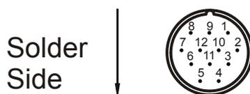
Fig.: 18: View on EnDat mating connector of the RC series (internal thread M23)
