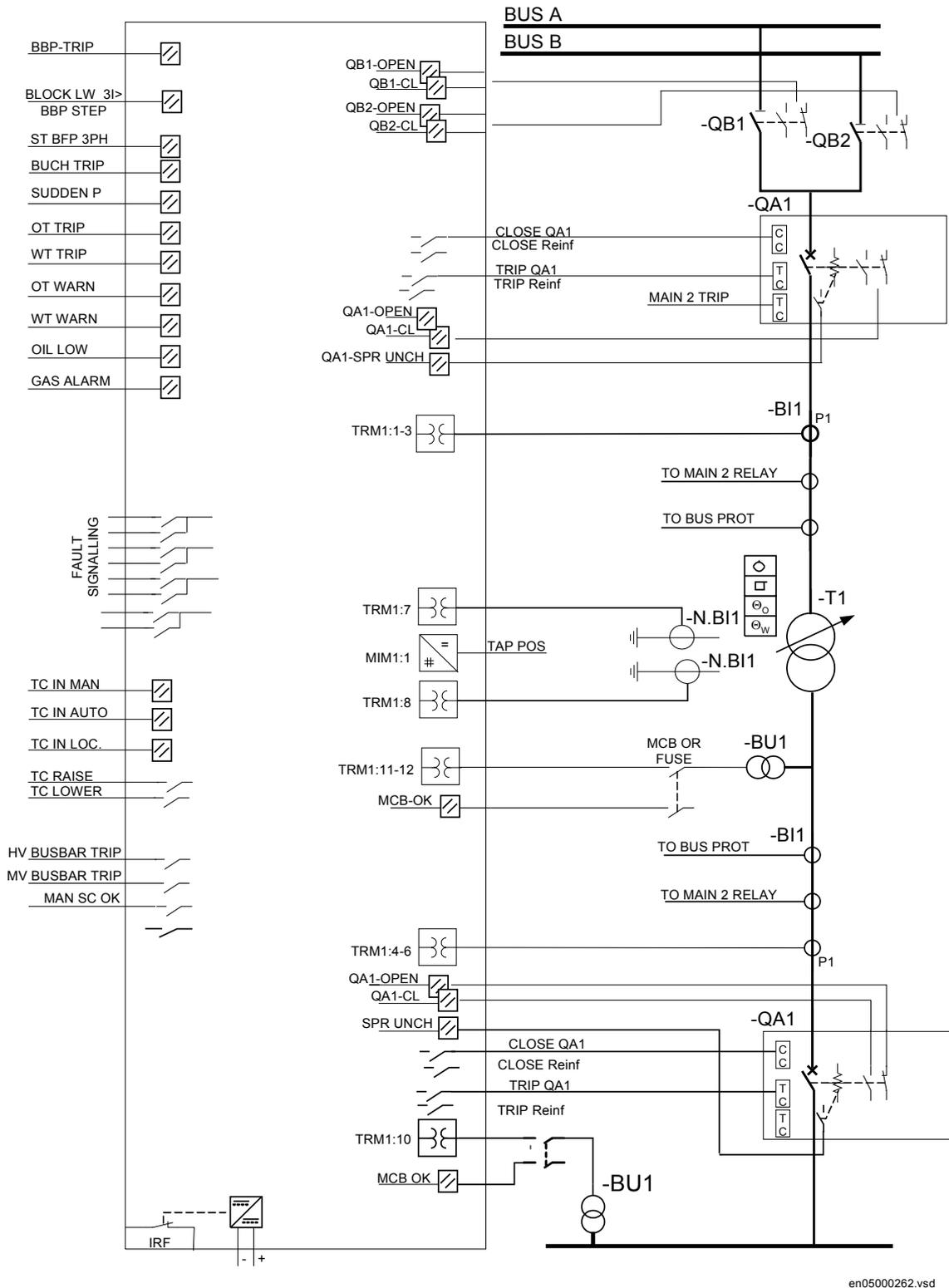
Figure 18. Typical connection diagram for two winding transformer in a single breaker arrangement. Note! Including IO for control option.
