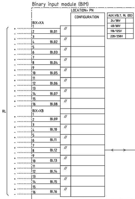
Figure 11. Binary input module (BIM). Input contacts named XA corresponds to rear position X31, X41, and so on, and input contacts named XB to rear position X32, X42, and so on.
