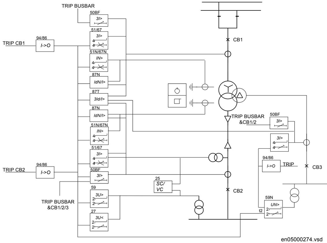
Figure 3. A typical protection application for a three winding transformer in single breaker arrangements is shown on the figure. The system earthing principle and connection group will vary which gives different detailed arrangements for each application.
