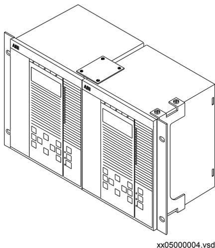
Figure 9. Side-by-side mounting
