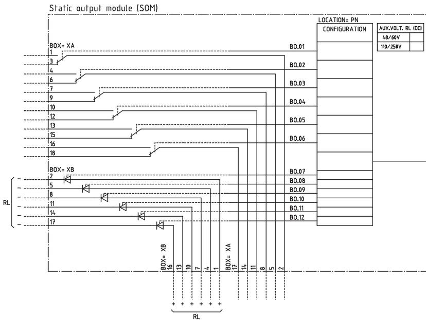
Figure 16. Static output module (SOM)
