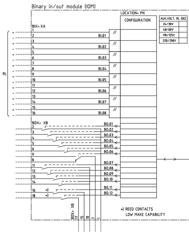
Figure 17. Binary in/out module (IOM). Input contacts named XA corresponds to rear position X31, X41, and so on, and output contacts named XB to rear position X32, X42, and so on.
