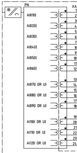
Figure 10. Transformer input module (TRM)
