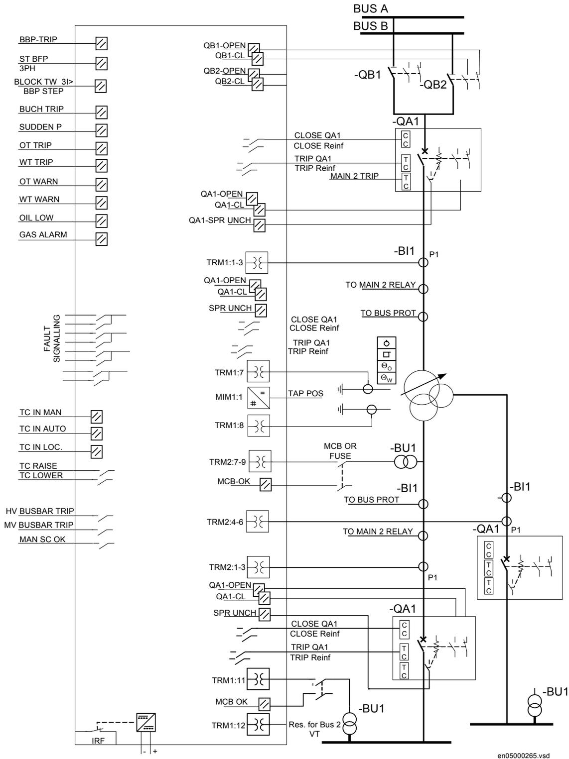
Figure 20. Typical connection diagram for three winding transformer in a single breaker arrangement. Note! Including IO for control option.
