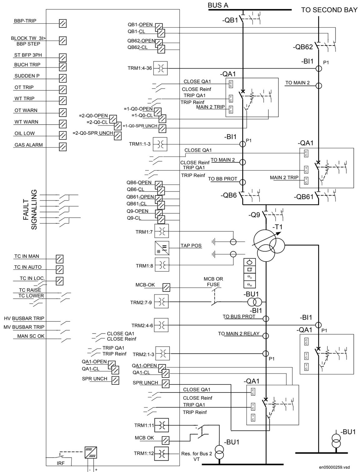
Figure 21. Typical connection diagram for three winding transformer in a multi breaker arrangement. Note! Including IO for control option.
