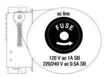
The power supply is protected from overcurrent at its inputs by a slow-blow fuse. The power supply comes with one 1A slow-blow fuse installed for 120V operation. If you are using the power supply for 220/240V operation, remove the 1A fuse and replace it with the 0.5A slow-blow fuse that is provided. Replacement fuses are shown below:
