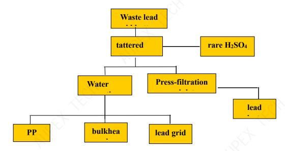
3.1.2. Explanation of the working principle of waste lead battery crushing and separation equipment
