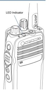
**Blinking yellow** – Radio is scanning for activity or receiving a Call Alert, or all local Linked Capacity Plus channels are busy.
