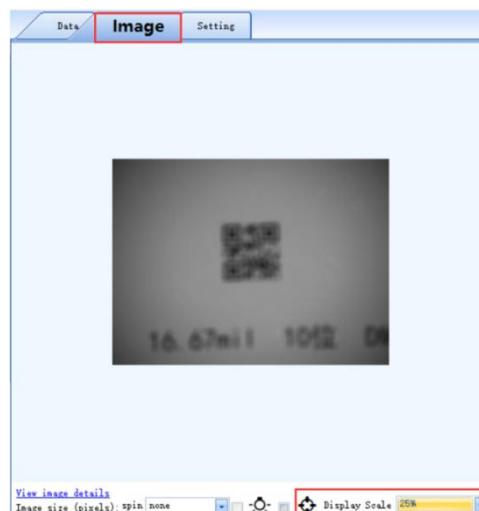
The captured image in the example is severely blurred, which affects decoding. It is necessary to adjust the focusing parameters of the reader. The display ratio can be adjusted according to needs.
