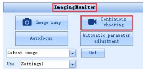
2.The current shot images are displayed in real time. If the image is blurred, use the attached hex wrench to adjust the focus tuning knob and check the real-time focusing status from the image until it is clear;
