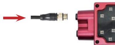
The arrow in the figure indicates the connection position of the Ethernet communication cable. Align the protrusion on the cable connector with the groove of the corresponding device port; Rotate the connector screw clockwise to secure it; It is prohibited to plug and unplug the connector during normal working state/configuring process, otherwise it may cause abnormal states of the reader to occur.
