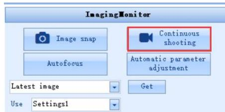
3. Check the real-time images captured; Place the barcode at the center of the Image interface, ensuring the barcode is in reader's field of view; Perform the focusing operation. For specific focusing operations, you can refer to the content in Chapter 6.2;
