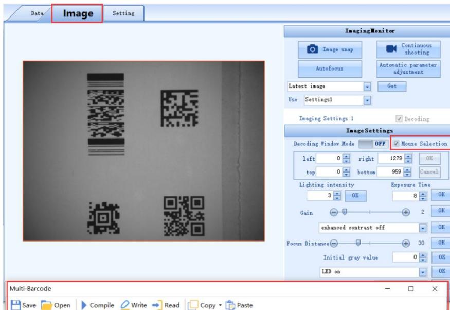
3. After selecting an area by mouse, the information of the selected barcode area will be automatically updated to the corresponding setting items in "Multi-Barcode" , click "Add sequence rules" , as shown in the figure:
