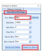
Click on "Connect to device", the interface is shown as follows after successful Serial port connection:
