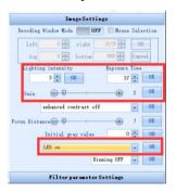
Fix the device at a certain height, click on Continuous Shooting, view the real-time image in the Image interface. Adjusting the data of "Lighting intensity", "Exposure time" and "Gain" while viewing the image. Keep adjusting until a green border appears around the barcode.
