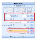
Fix the device at a certain height, click on continuous shooting, view the real-time image in the image section. Adjusting the data of "Lighting intensity", "Exposure Time" and "Gain", view the image while adjusting. Continuously adjust until the barcode image is clear and a green box appears.
