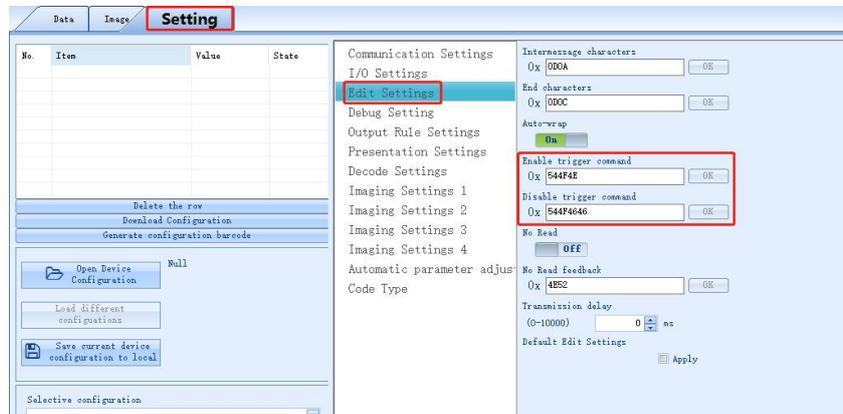
2. Set the trigger command, for example, set "LON" as the trigger command, select "Transformation Assistant", and input "LON" to convert "LON" to the corresponding hexadecimal;
