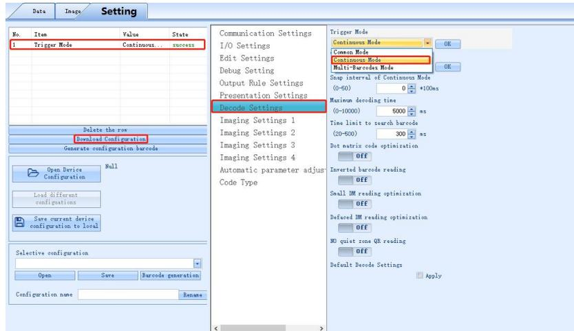
2. The startup mode of continuous trigger mode is divided into boot startup and I/O trigger. The default is I/O trigger.
