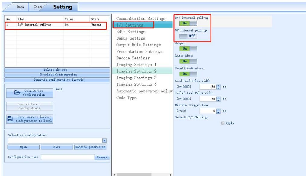
2. IO output logic, OUT1-OUT2 output level signals are all 24V.
