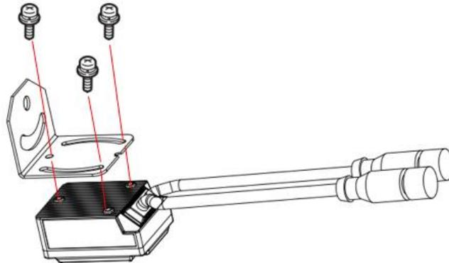
Use the mounting bracket to obtain the most appropriate reading position. The figure shows the most common installation configuration. The installation position of L-type metal fixing plate can be adjusted according to the actual needs.
