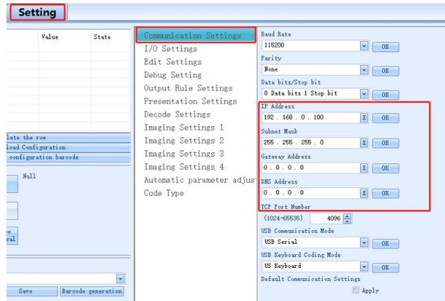
2. "IP address", "subnet mask", "gateway address", "DNS address" and "TCP port number" can be set according to requirements. Take the IP address as an example, the IP address can be directly entered by keyboard according to requirements;
