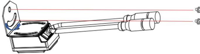
As shown in the figure, adjusting the angle of the equipment to the appropriate angle position, and fixing the L-shape firmly with screws.
