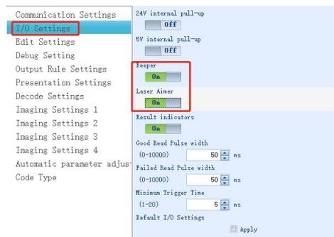
1. When the FV5X code reader succeeds or fail in reading the code, the buzzer and the laser aiming functions are open by default;
