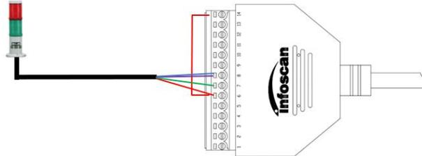
The device defaults to the initial logic and connecting pin 14 (24V) of the 14pin terminal to the com-in terminal. Meanwhile, the positive pole of the load (taking the NPN alarm lamp as an example) is connected to the com-in terminal and the negative pole is connected to the out1 or out2 in output terminal. When reading is successful, the green light is on, and when reading fails, the red light is on and the alarm sounds. The corresponding table of line sequence is as follows:
