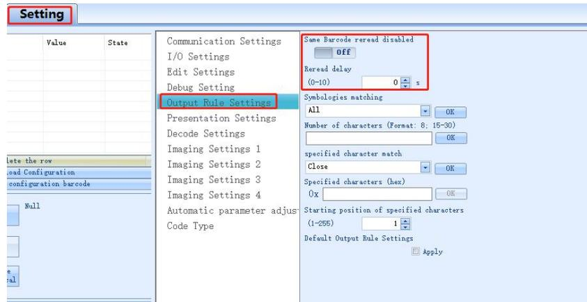
2. FV5X barcode reader repeat barcode reading is set active, repeat reading delay time is set to "5".
