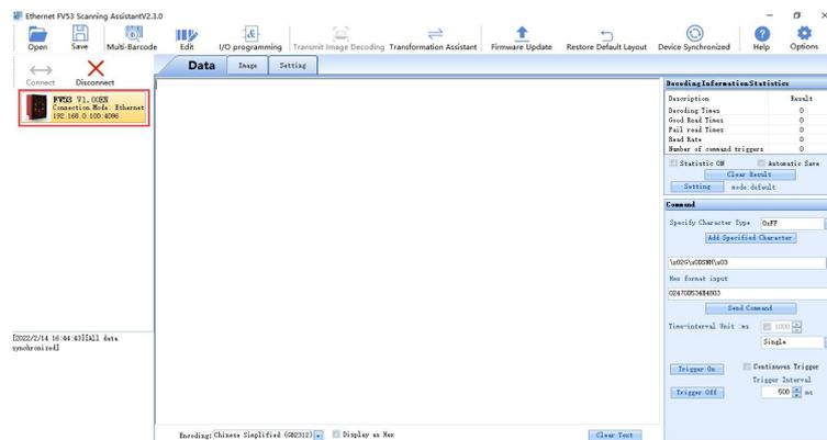
**Note:** Display online device model and version information and connection method, device IP address and port number information; the feedback information part displays the date and time of the connection and other related information; after the connection is successful, the interaction is successful, you can click "Image" or "Setting" "Make relevant detailed settings for the barcode reader.
