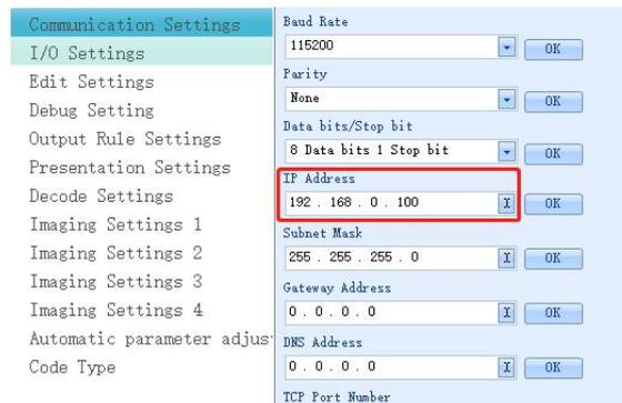
3. After the IP address input is completed, click the "Confirm" button, the set IP address will be displayed in the list, click the "Set Download" button, the buzzer of the code reader will prompt that the setting is successful, and the setting status is displayed successfully, that is, the setting is successful;
