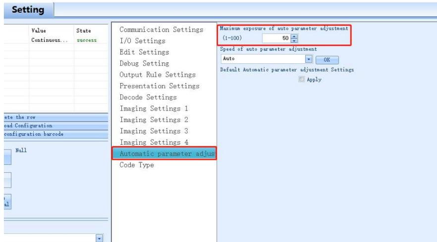
2. Automatic parameter adjustment speed: The default is automatic (self-adaptive), Automatic, high-speed, medium-speed, and low-speed can be selected.
