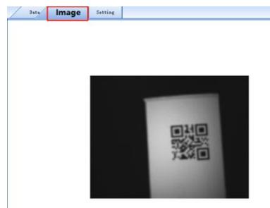
The sample captured image is blurry, which affects decoding, then the focus parameters of the code reader need to be adjusted.
