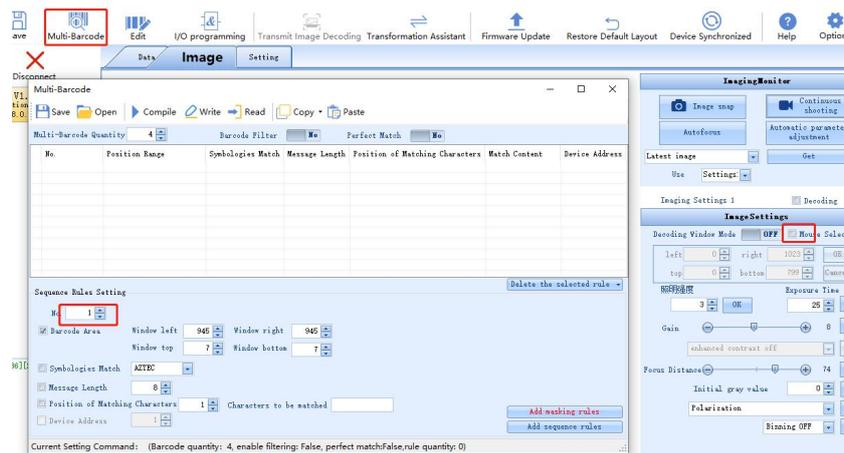
After selecting the box with the mouse selection function, the current address information will be automatically updated to the multiple barcode rules, as shown in the figure:
