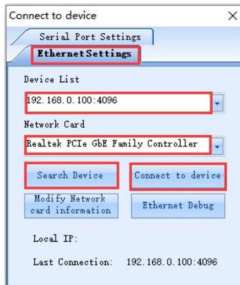
Click "Connect to device" after the connection is successful, the device will have a buzzer prompt, as shown in the figure:
