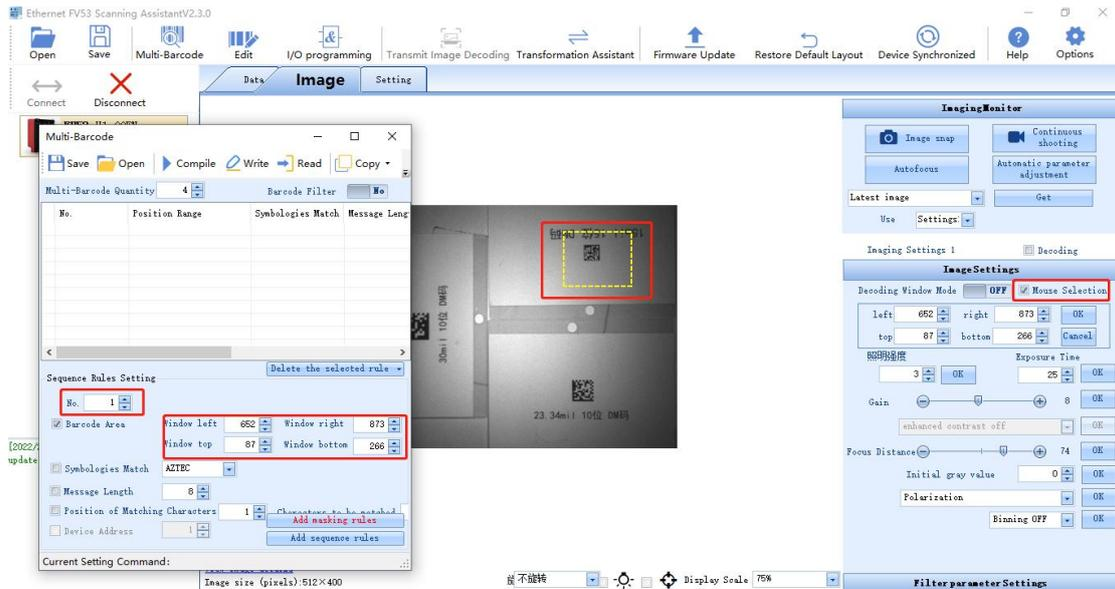
To set the second barcode, set the output sequence to 2, and re-select the box to select a new address.
