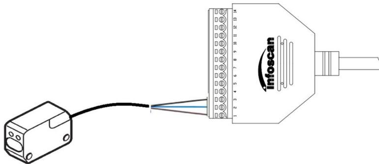
The equipment defaults to the initial logic. The photoelectric sensor shall be NPN type, and the photoelectric sensor shall be connected to signal terminals 1, 2 and 3. The corresponding line sequence is shown in the table:
