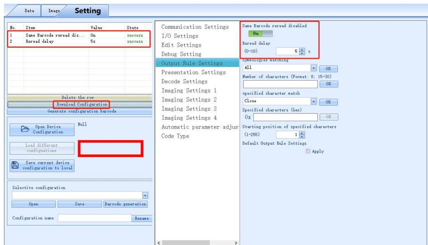
3. The repetition reading time is set to 5s, and the repetition barcode reading function is kept for 5s.
