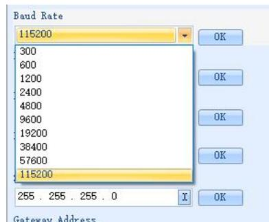
3. Click "Download Configuration", if the setting is successful, the barcode reader buzzer will give feedback, then the setting status in the list will display "Success", indicating that the baud rate setting is successful.
