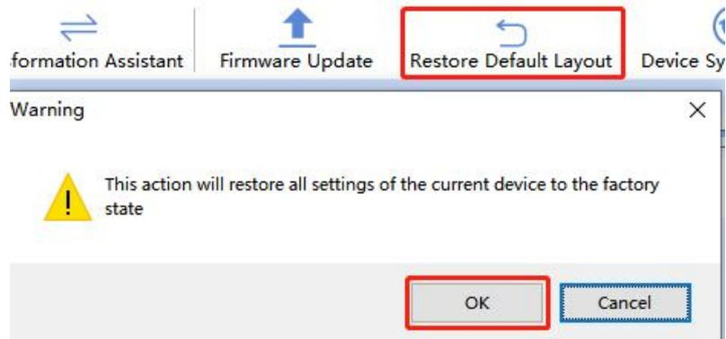
After hearing the device beep and seeing the success message, the device has been restored to the factory state successfully.
