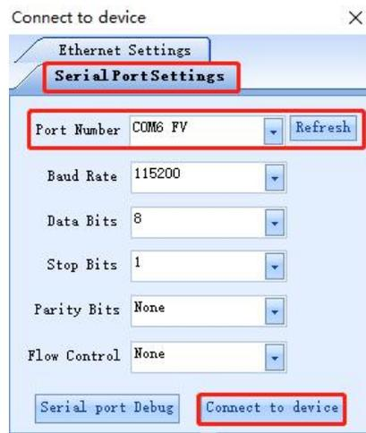
Finally click "Connect to device", The USB connection screen is as shown in the figure:
