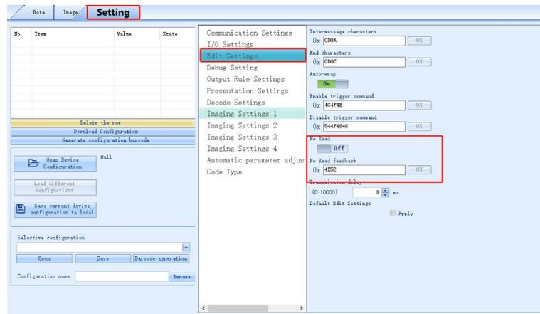
2. The read failure feedback switch is set to on, and the read failure character feedback character (hex) is set to "NoRead". Use the conversion assistant to convert "NoRead" to hexadecimal, paste the hexadecimal content into the read failure character feedback character, click "OK", view the list, click "Download Configuration" to complete the setting.
