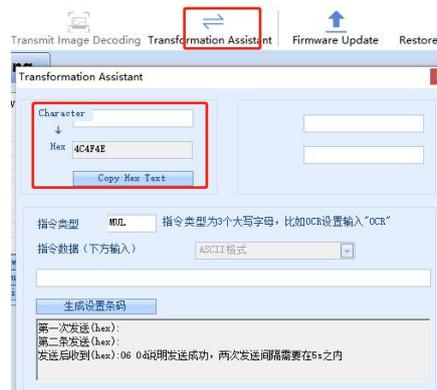
3. Copy the Hex content converted by "LON", paste it into "Enable trigger command", click "OK", you can view it in the setting list, click "Download Configuration" to complete the setting;
