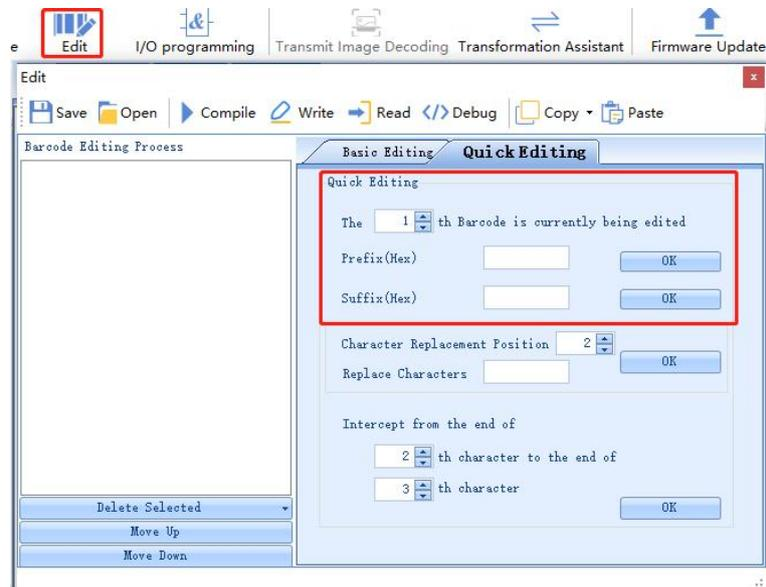
You can enter the required characters in the text boxes after the prefix and suffix. The input text is in hexadecimal, which can be converted by the conversion assistant. If you want to add "ABC" characters before and after the barcode, open the conversion assistant, enter "ABC", it will be automatically converted to hexadecimal, click to copy the hexadecimal text.
