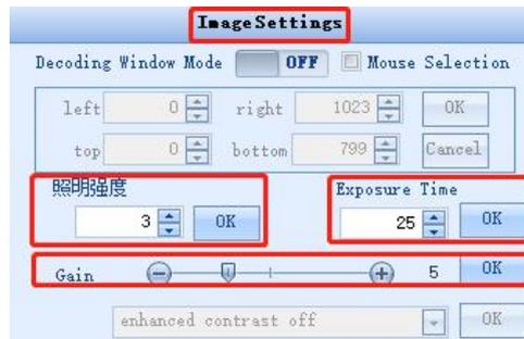
2. Adjust "照明强度", "Exposure Time" and "Gain" to view the image changes in real time, as shown in the example. When the illumination intensity is set to 0, the image is dark, while the illumination intensity is set to 2, the image is obviously brighter and the sample barcode is displayed in a green frame, which can be successfully decoded;
