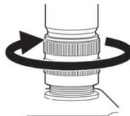
3. After the aviation cable plug (male) is firmly connected with FV5X, then the serial communication cable DB9 (female) is connected to the PC serial port, and the Ethernet communication cable RJ45 is connected to the PC Ethernet port (see computer wiring for details).
