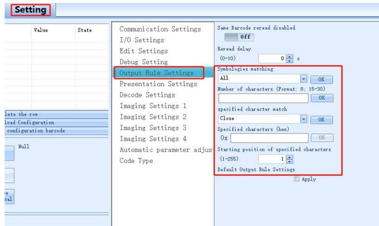
2. For example, if the output code system is QR barcode, the number of characters is 10, and the settings are as follows.
