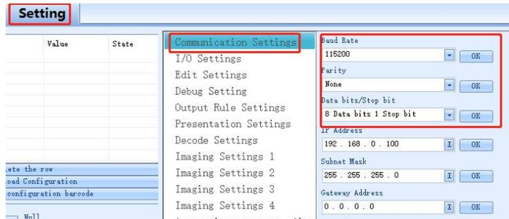
2. "Baud Rate", "Parity" and "Data bits/Stop bits" can all be set according to requirements. Take the baud rate setting as an example, set the baud rate to 9600, select "9600" and click the OK button.
