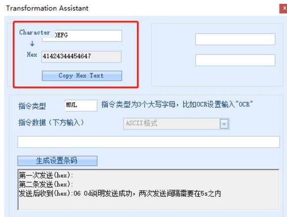
Paste the copied hexadecimal text into the corresponding prefix character input box in the barcode editor. Confirm, compile, write.
