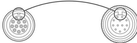
2. Rotate the aviation plug (male) screw clockwise to fix it.
