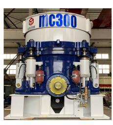
MC Multicylinder cone crusher
