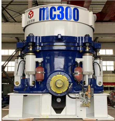
MC Multi-cylinder cone crusher
