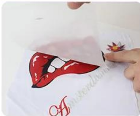
Peel Off PET Film Carefully
