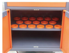
■ 柜子内部有一层刀套板，可放刀柄 Double drawer with partition on top
