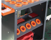
下面配置两条外倾式刀柄架 There are two extroverted toolholders
