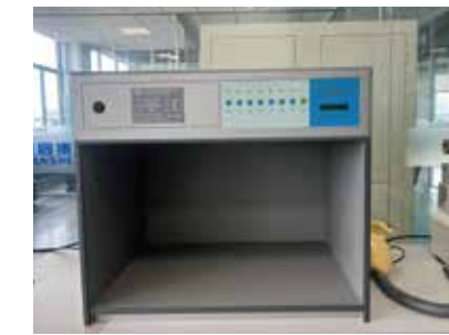
Standard Light Source Color Matching Light Box
