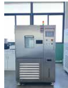
Constant Temperature and Humidity Test Chamber
