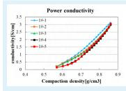
Parameter: relief mode: 10~200MPa, 10MPa steps, keep 10s Results: The cov of five parallel samples is less than 0.3% in the whole pressure range, which indicates that **the equipment** has good repeatability.
