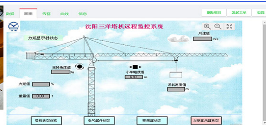
Remote monitoring platform and Mobile terminal
