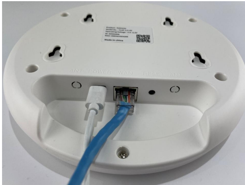
Figure 3-3 Power and network cable connection example
