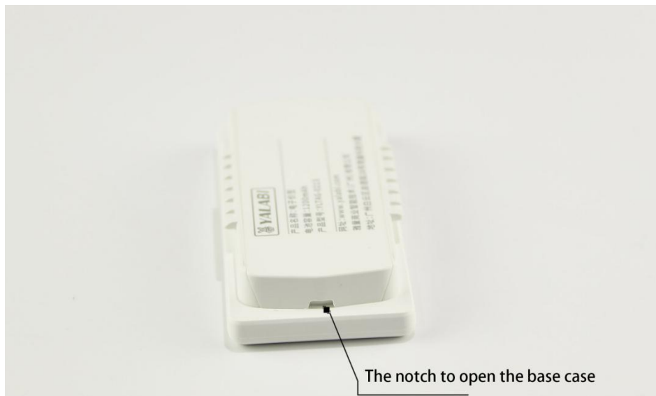
Figure 2-8 The notch to open the base case
