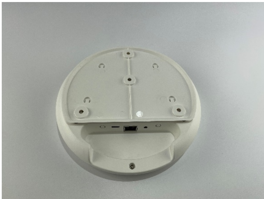
Figure 3-2 Ceiling installation of base station
