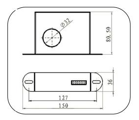
Passive Lightning event counter is used for registering the direct lightning event.
