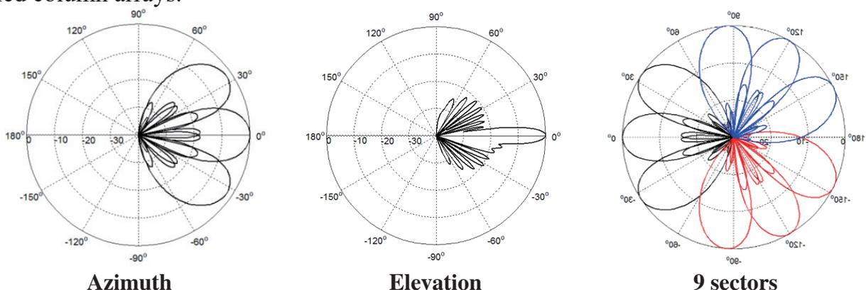
**Figure 3** patterns of triple beam antenna
