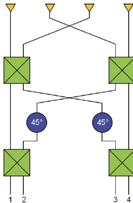
**Figure 2** The architecture of the sector-sculpting Twin Beam antenna
