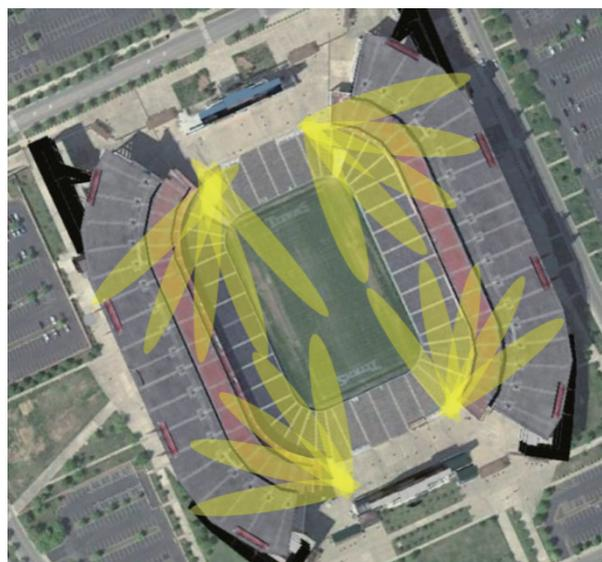
**Figure 10 Stadium huge data solution with 4 penta beam antenna**
