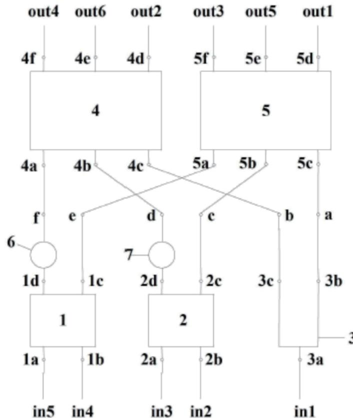
**Figure 8** The architecture of the sector-sculpting Penta Beam antenna
