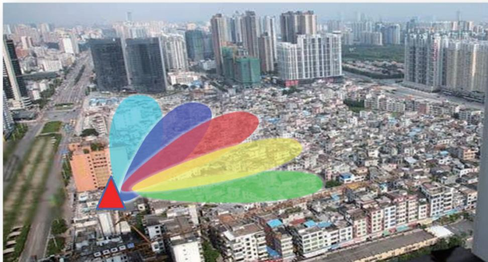
**Figure 9 High density area using penta-beam antenna coverage**
