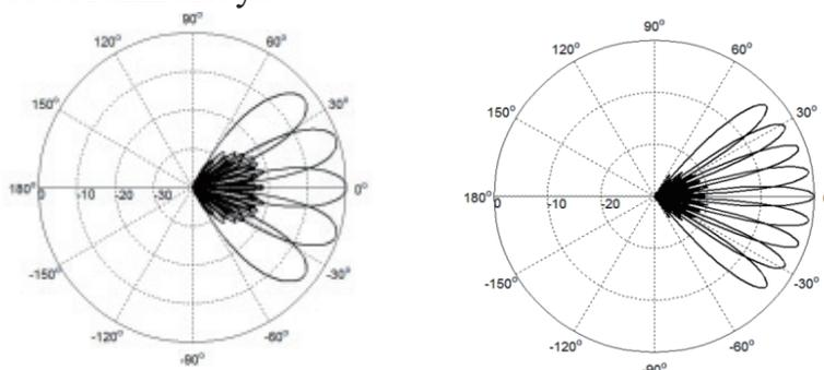
**Figure 7 Multi-beam transmit patterns.**
