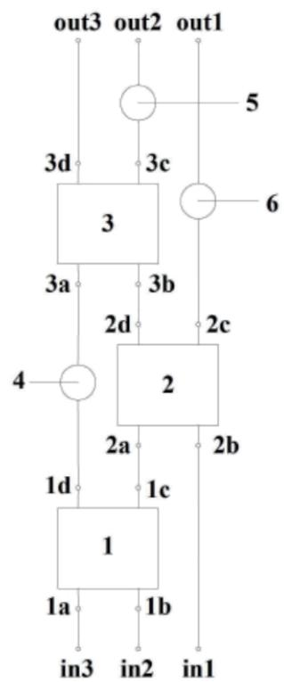
**Figure 5** The architecture of the sector-sculpting Triple Beam antenna
