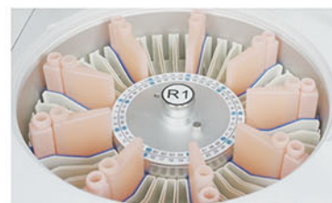
Reagent Tray 2~8°C cooling for 24 hours.
