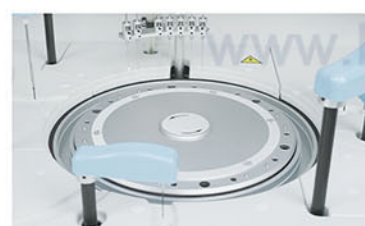
Reaction Tray 37±0.1°C, real-time monitor.
