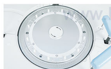
Reaction Tray 37±0.1°C, real-time monitor.
