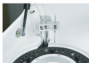
Washing Probe Independent 3 -step washing system.
