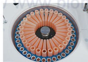
Reagent Tray Refrigerated tray with independent switch.
