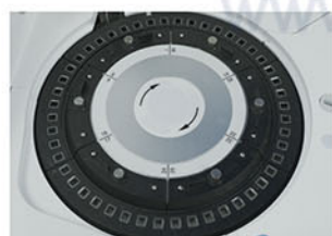
Reaction Tray 37±0.2°C, real-time monitor.
