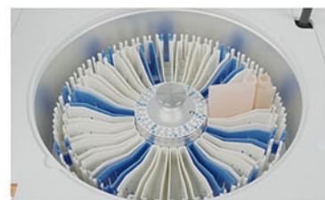
Reagent Tray 2~12°C cooling for 24 hours.
