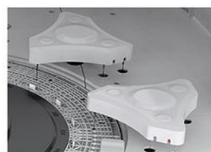
Mixer Probe Dual mixer, auto frequency adjustment.
