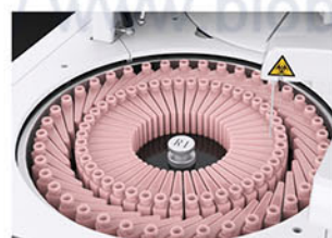
Reagent Tray 2~8°C cooling for 24 hours.
