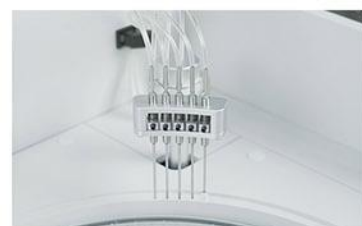
Washing Probe Independent 5-step washing system.
