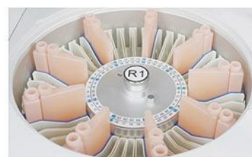
Reagent Tray 2~8°C cooling for 24 hours.
