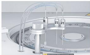
Washing Probe Independent 3-step washing system.
