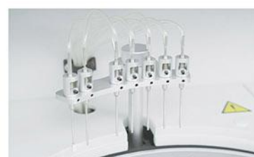
Washing Probe Independent 7-step washing system.
