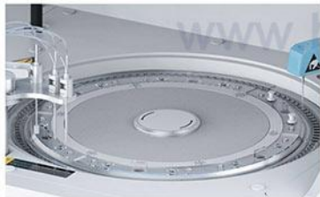
Reaction Tray 37±0.2°C, real-time monitor.
