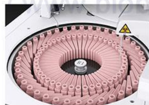
Reagent Tray 2~8°C cooling for 24 hours.
