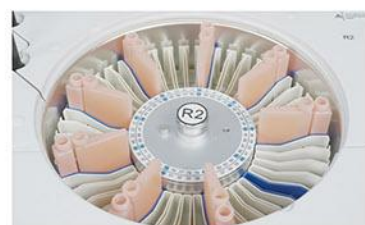
Reagent Tray 2~8°C cooling for 24 hours.
