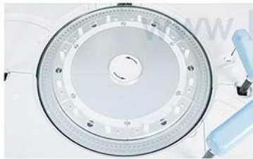
Reaction Tray 37±0.1°C, real-time monitor.
