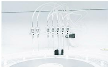
Washing Probe Independent 7-step washing system.
