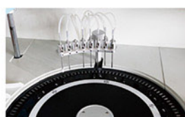
Washing Probe Independent 7-step washing system.
