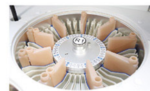
Reagent Tray 2~8°C cooling for 24 hours
