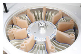
Reagent Tray 2~8°C cooling for 24 hours.
