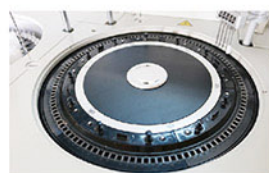
Reaction Tray 37±0.1°C, real-time monitor.
