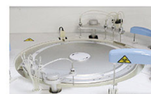
Reaction Tray 37±0.1°C, water bath
