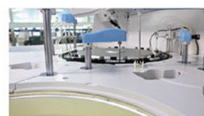
Mixer Probe Dual mixer, auto frequency adjustment
