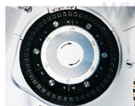
Reaction Tray 37±0.2°C, real-time monitor.
