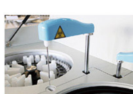
Sample Needle Liquid level sensor function. Anti-collision function. Reagent volume real-time detection.
