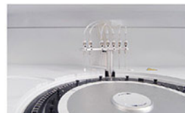
Washing Probe Independent 7-step washing system.
