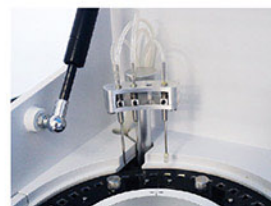
Washing Probe Independent 3-step washing system.
