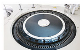
Reaction Tray 37±0.2°C, real-time monitor.
