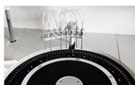
Washing Probe Independent 7-step washing system.
