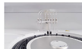
Washing Probe Independent 7-step washing system.
