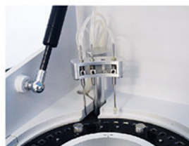
Washing Probe Independent 3-step washing system.
