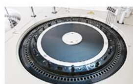
Reaction Tray 37±0.2°C, real-time monitor.
