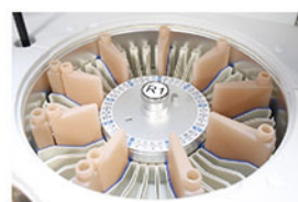
Reagent Tray 2~8°C cooling for 24 hours.
