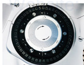
Reaction Tray 37±0.2°C, real-time monitor.
