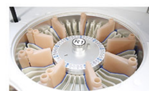
Reagent Tray 2~8°C cooling for 24 hours
