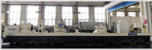
**Equipment: CNC deep hole drilling and boring machine**
