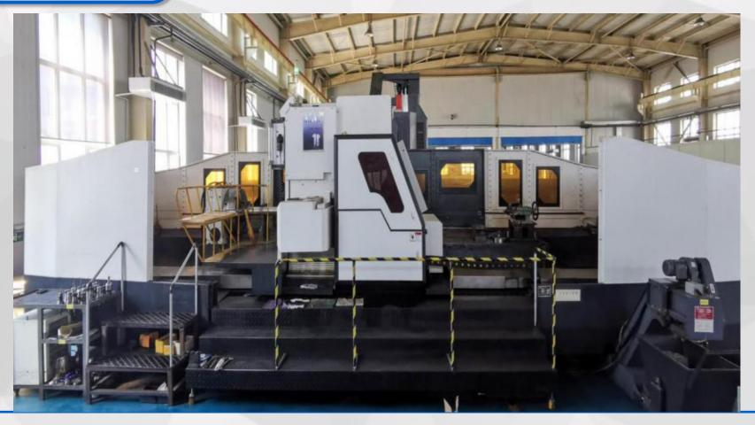
**Euipment: Horizontal CNC boring and milling machine**
