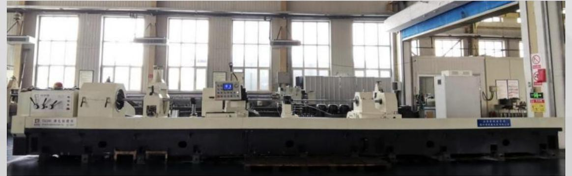
**Equipment: CNC deep hole drilling and boring machine**
