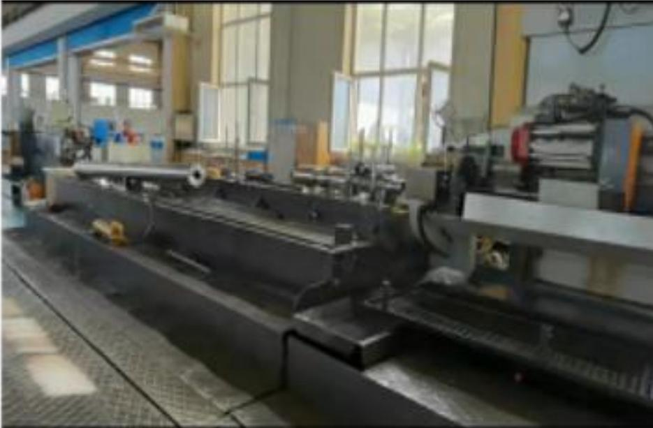
**Three-coordinate CNC deep hole gun drill**
