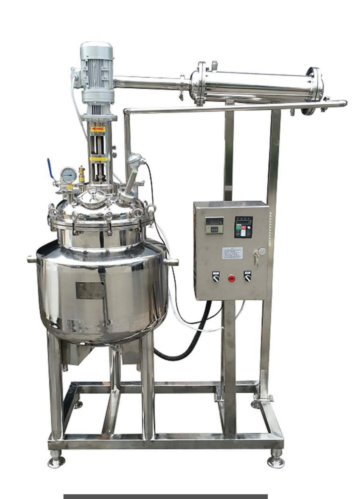
带冷凝的反应釜 Reactor with condensation
