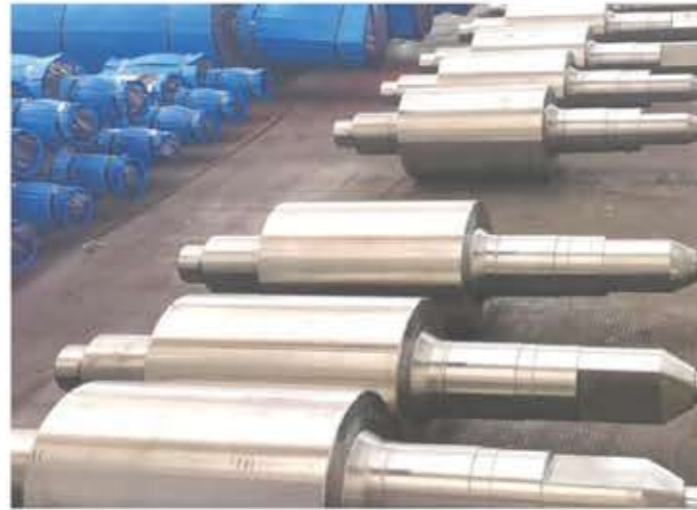
rolls for rebar
