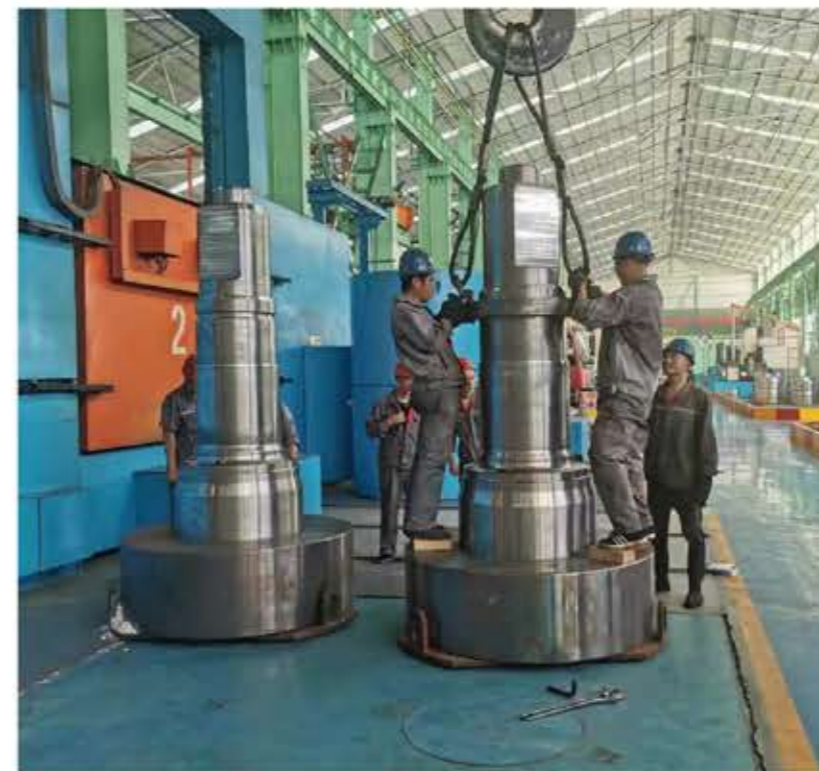
section mill rolls under installation
