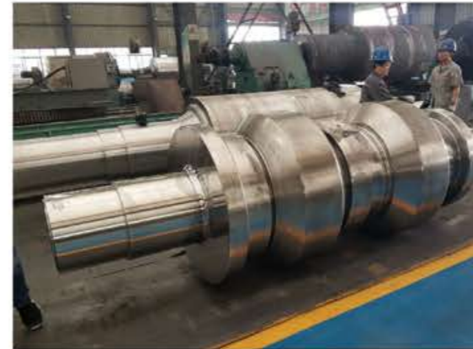
Steel sheet pile rolls
