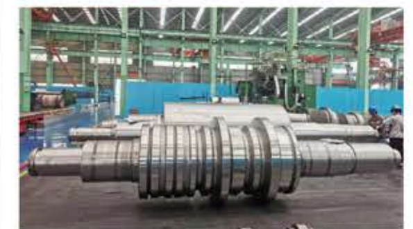
section mill rolls
