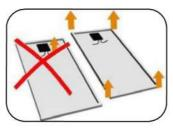
Carry modules with both hands. Do not use the connection socket as a handle; Don't lacerate the frame during handling and installing.
