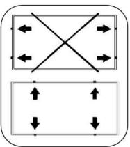
Each module should be fixed at least 4 points on long frame or short frame.
