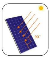
In order to achieve maximum annual yield, optimum orientation and tilt of PV modules is necessary. Sunlight shining vertically onto the PV module is the best condition to generate maximum power.
