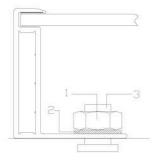
Use the existing installation holes instead of drilling additional holes for installation (Drilling holes shall against the reliability and warranty of the modules). The installation and attachment materials (nuts, bolts, etc) must be corrosion-resistant. Moment of force is 5N • m for module mounting.
