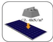
The maximum load on module must not exceed 2.4KN/m<sup>2</sup>. Site-specific environment loads such as wind and snow should be taken into account to avoid exceeding the maximum
