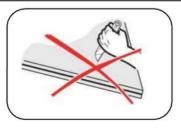
Do not mark on the rear of the module using sharp objects.
