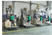
立式注塑机 Vertical Injection Molding Lines
