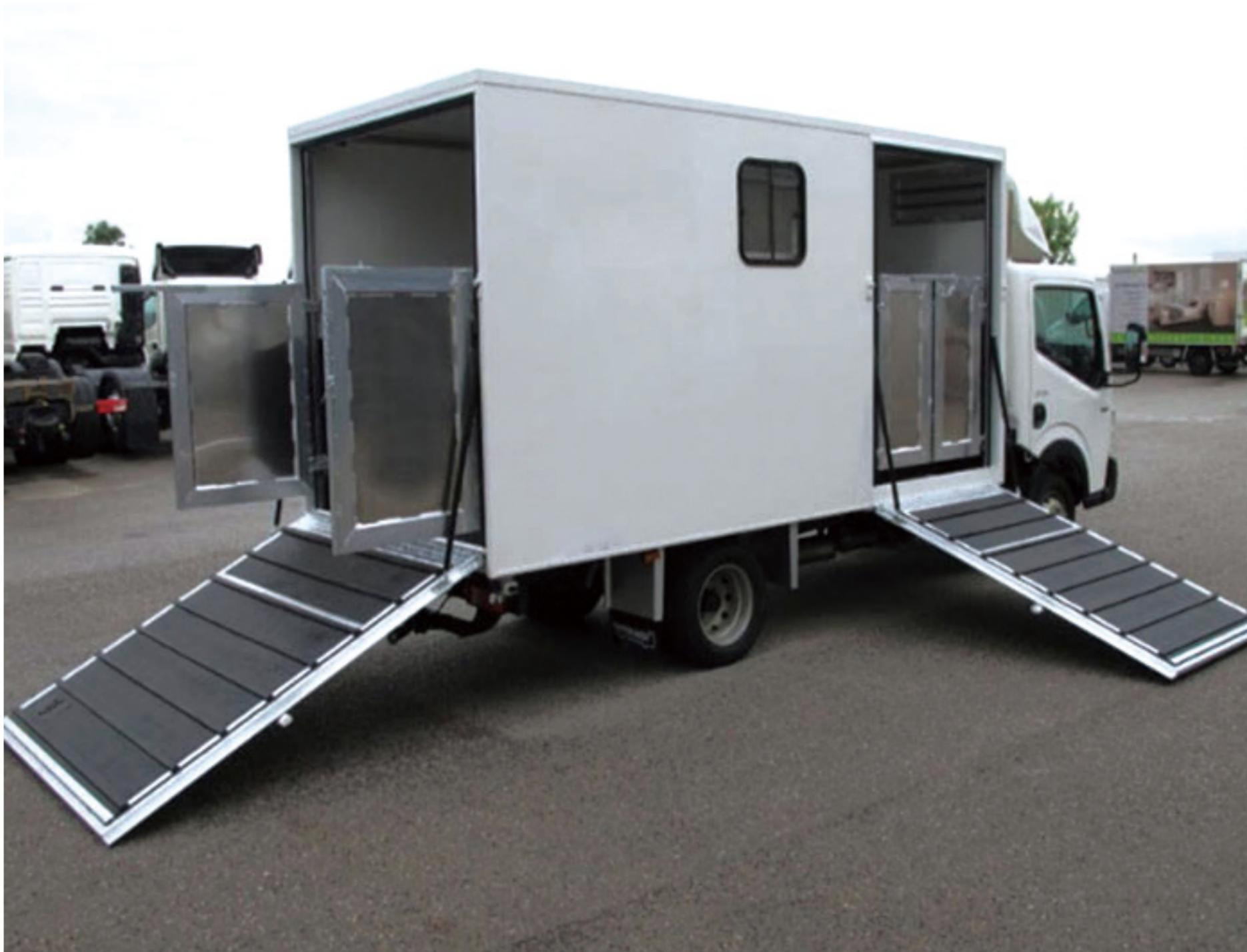
Aluminum honeycomb panel, is suitable for for vehicle, electric ramp.
