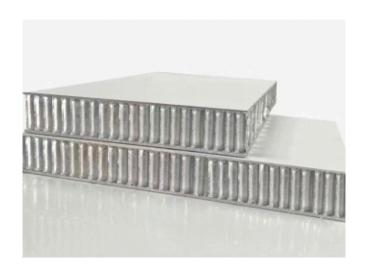
This honeycomb panel is sandwich structured composites comprising of aluminum honeycomb core and two skin sheets in mill finish, bonded together by aviation grade adhesive film that can resistant temperature up to 200 °C. The panel can be processed to custom size and special shape, as well as be welded and sanded to meet the industry design.
